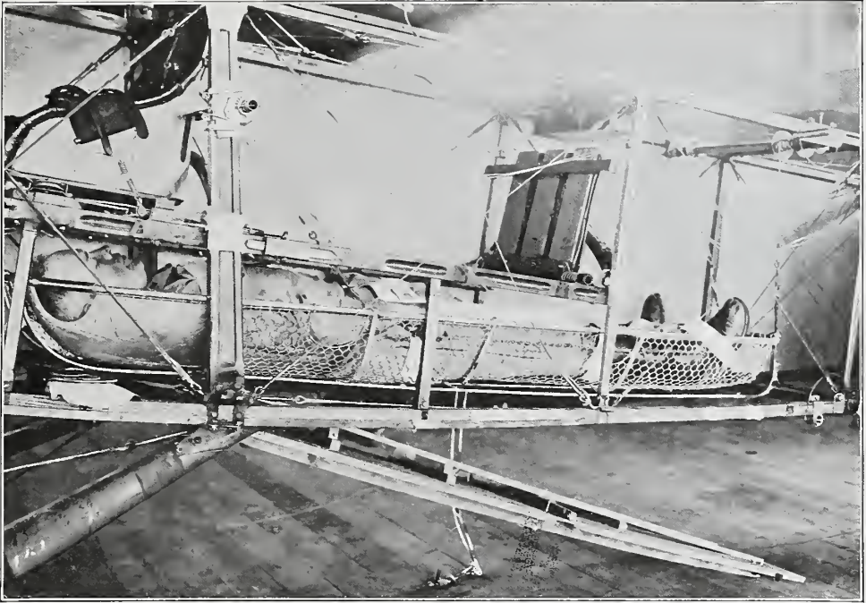
FIG. 148.—Winching Stokes litter into place in the Rockwell Field airplane ambulance.
